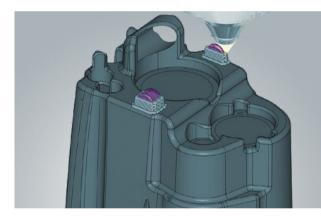
The user can access all of the hyperMILL® machining strategies for the subsequent machining of the two features. The programming of the material application and removal takes place within the same user interface, and it is output using the same postprocessor. In addition, hyperMILL® ensures programming continuity from the simulation right through to the stock chains.
