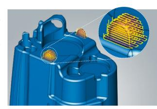
2 The material for the two new features is applied using the DED hybrid milling machine. In the subsequent subtractive machining job, the simulated material application also serves as a stock model, which means it is included in the collision check.
