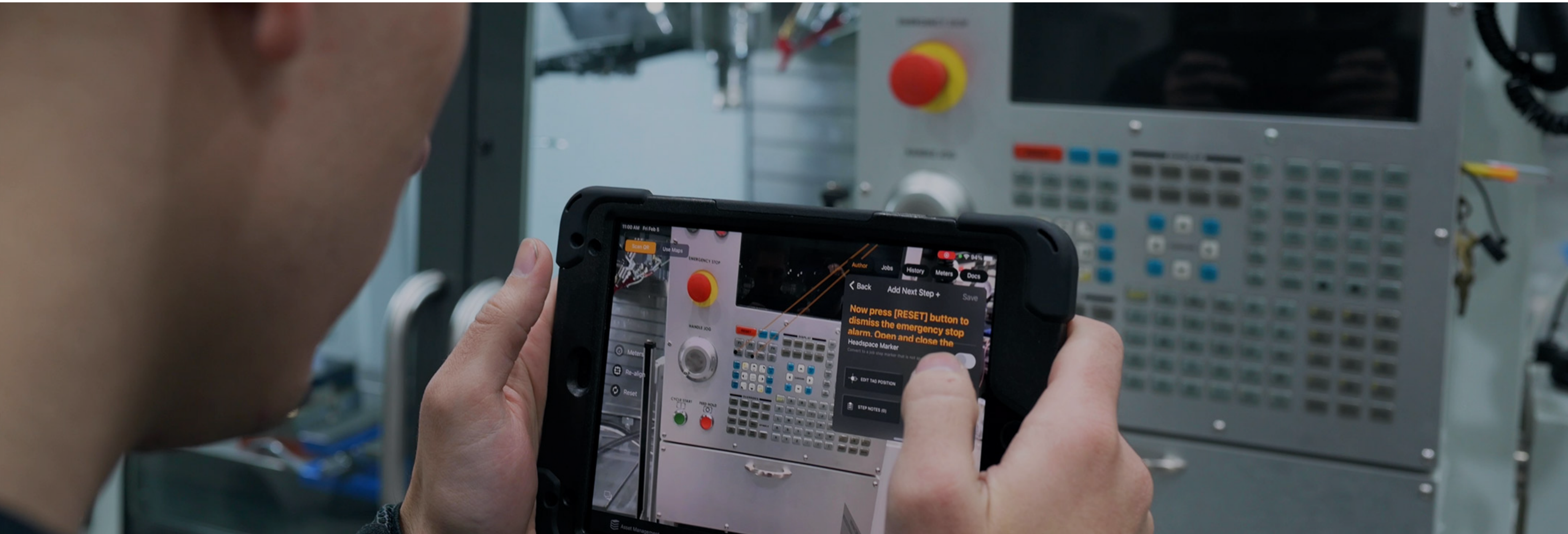
Image 1: iPads are used to create spatial markers that associate instructions with a specific location on a machine.
