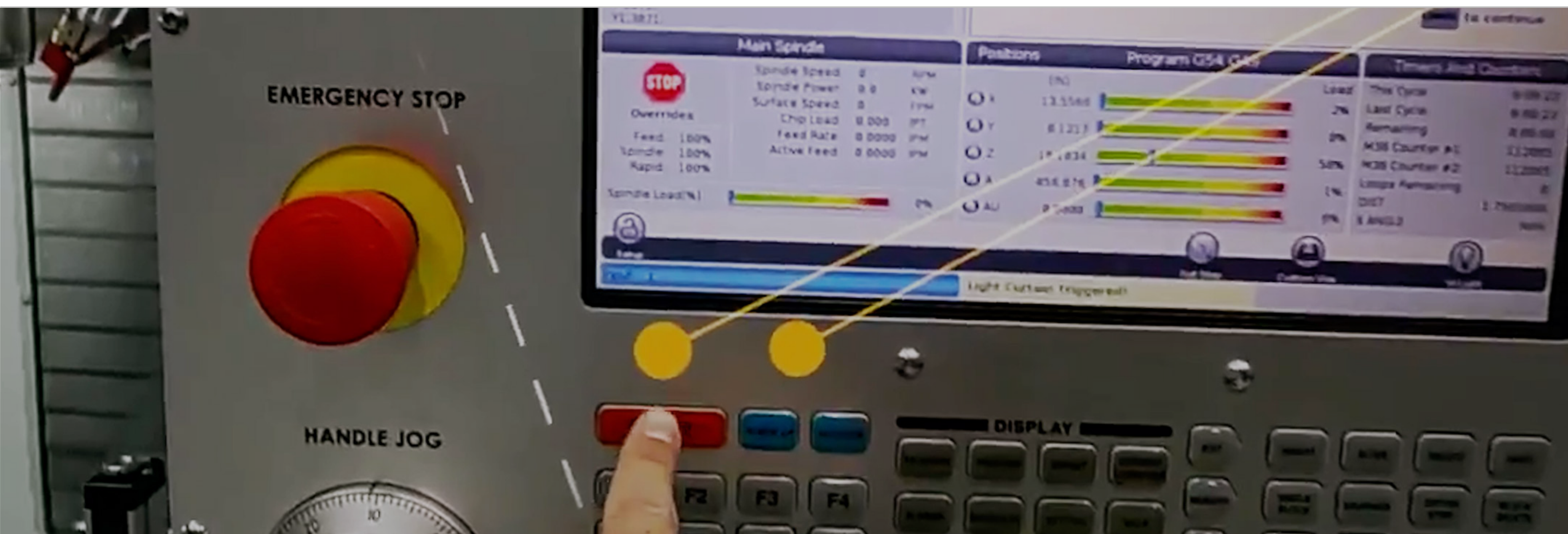
Image 2: Spatial markers associated with instructions show operators which buttons to use to perform a procedure.
