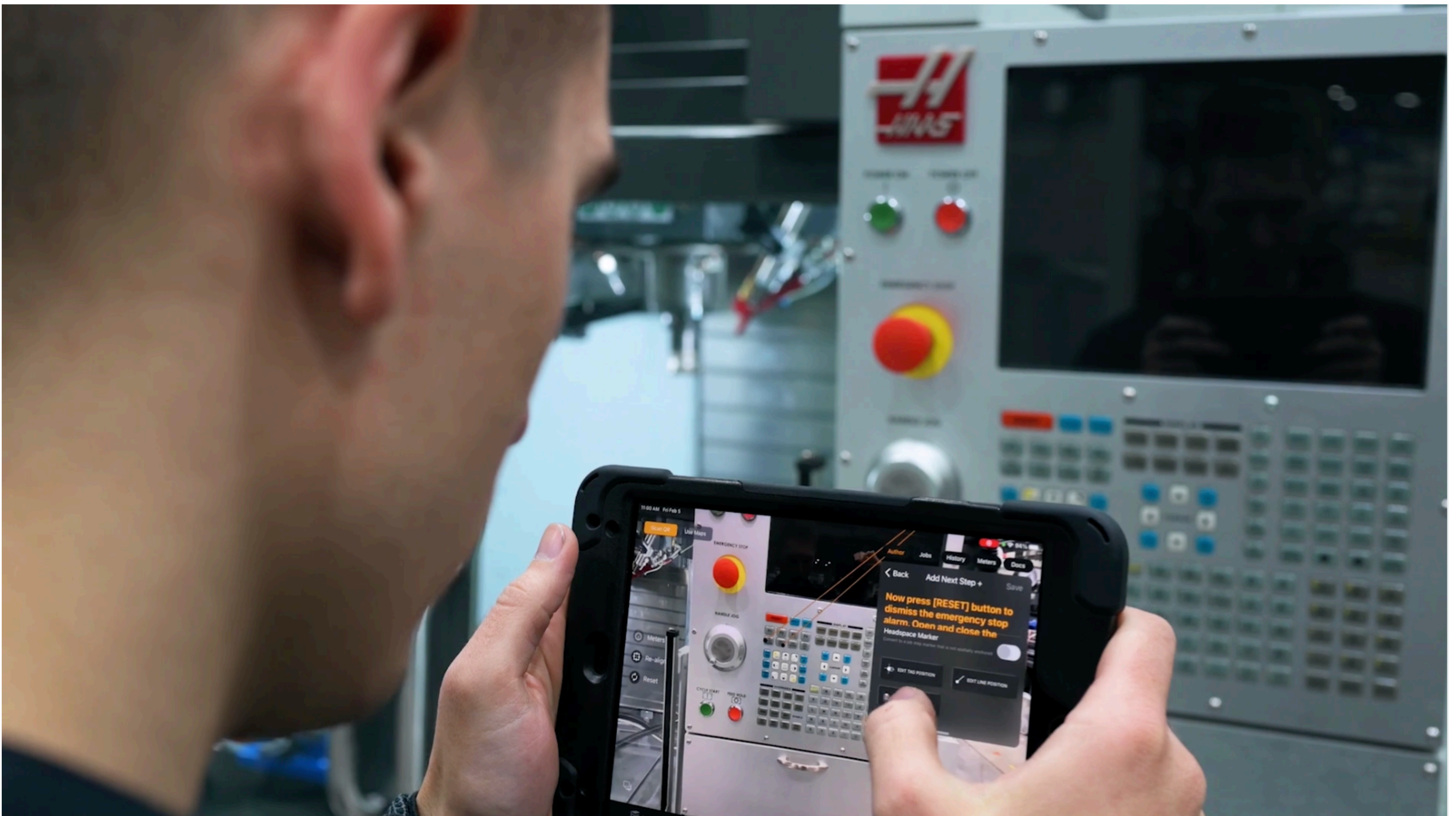
Manifest utilizes spatial markers associated with instructions to show technicians where to perform a procedure.
